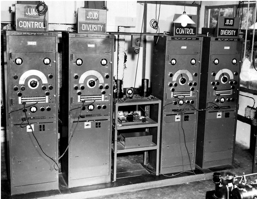
North Africa, 1944. Two pairs of RC67 receivers connected in dual diversity.
