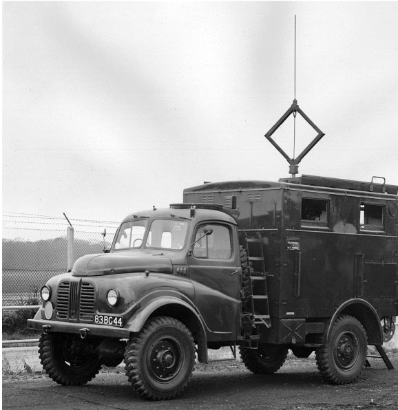
DF Station Mobile B/C No. 2A in Truck 1-ton GS Wireless Light (Austin K9)
